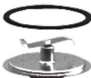
Place the seal on the rim of the blade assembly, making sure it is completely flat.
