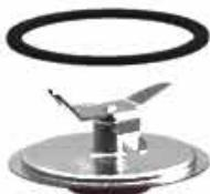
Place the seal on the rim of the blade assembly, making sure it is completely flat.
